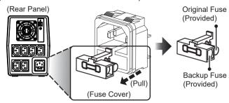
Replace the original fuse with the provided backup fuse 2.
