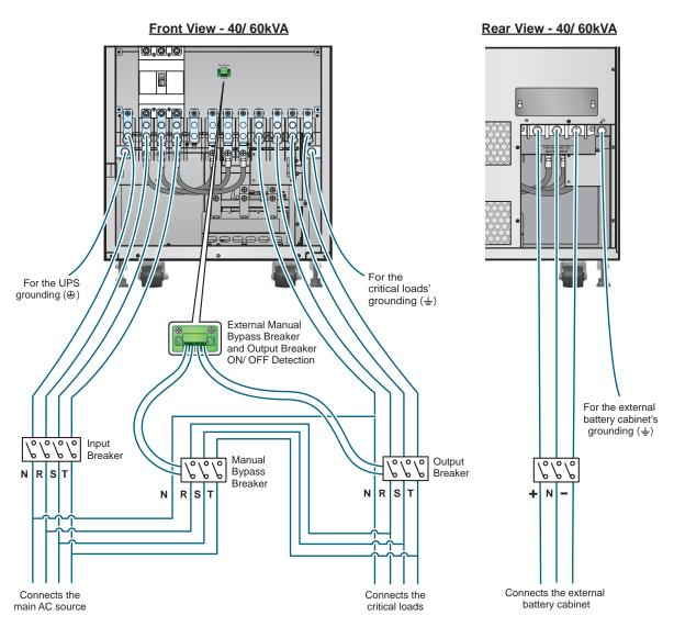
(Figure 5-10: Single Unit Single Input Wiring Diagram\_40/60kVA)
