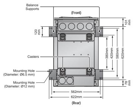
(Figure 5-1: Mounting Hole Diagram)
