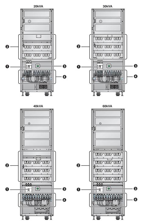
(Figure 3-10: Front View with Door Open and Internal Panel Removal (Models without Internal Batteries))
