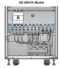
(Figure 5-5: Three Cables Location)
