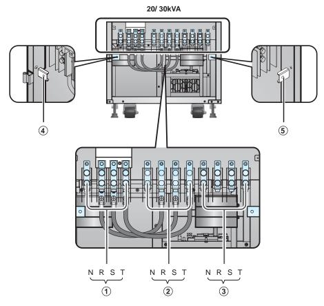
(Figure 3-8: Wring Terminal Block\_20/30kVA)
