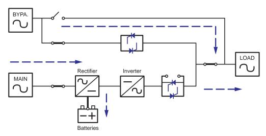
(Figure 4-5: Path of Electrical Power through the UPS in Bypass Mode)
