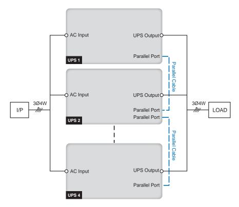
(Figure 5-14: Parallel Units Single Input Wiring Diagram)
