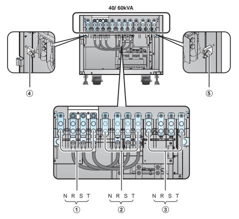
(Figure 3-9: Wring Terminal Block\_40/60kVA)
