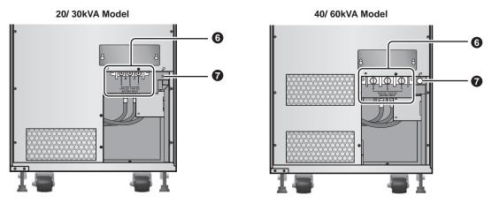
(Figure 5-8: Rear View\_Wring Terminal Block - 20/ 30/ 40/ 60kVA)
