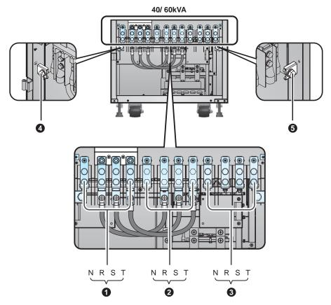
(Figure 5-7: Front View\_Wring Terminal Block\_40/ 60kVA)
