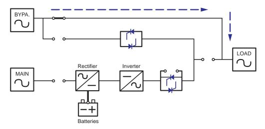
(Figure 4-6: Path of Electrical Power through the UPS in Manual Bypass Mode)
