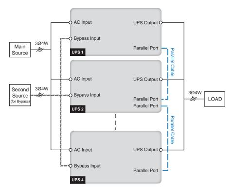
(Figure 5-15: Parallel Units Dual Input Wiring Diagram)
