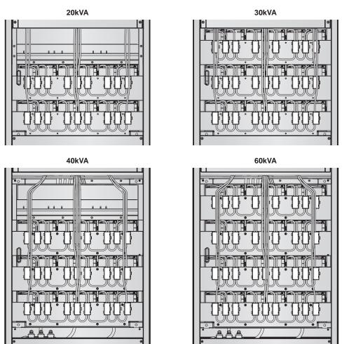
(Figure 5-11: Internal Battery Installation and Wiring)
