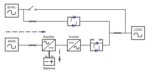
(Figure 4-2: Path of Electrical Power through the UPS in Standby Mode)
