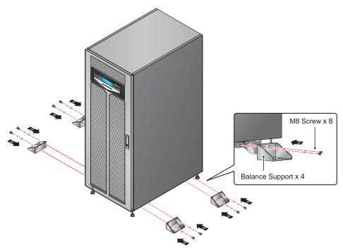
(Figure 5-2: Balance Support Installation)
