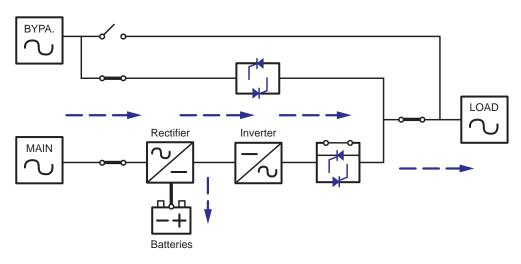
(Figure 4-1: Path of Electrical Power through the UPS in Online Mode)
