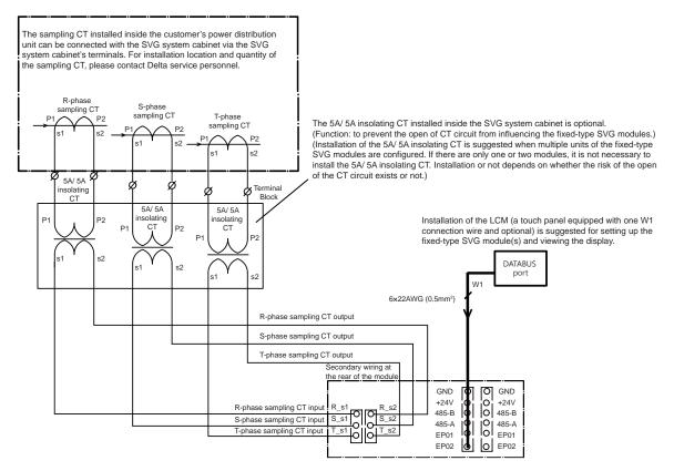
(Figure 3-8: Wiring Connection between the Rear of the Fixed-type SVG Module and the CT)
