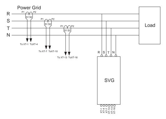
(Figure 3-14: Basic CT Installation and Wiring Diagram\_1)
