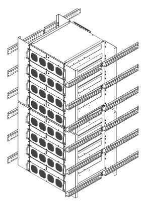
(Figure 3-9: Fixed-type SVG Modules & SVG System Cabinet Installation Diagram)
