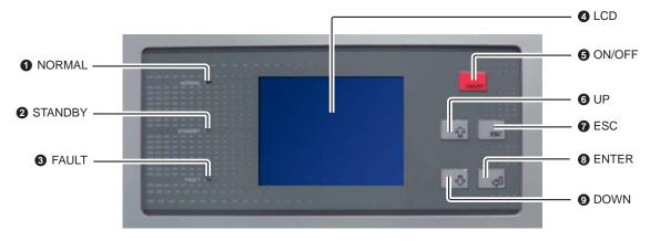
(Figure 2-4: LCM\_ Front View)
