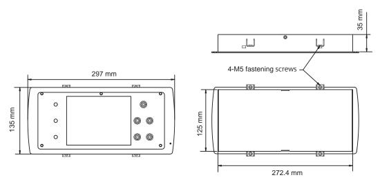
(Figure 3-5: LCM Structure and Dimensions)
