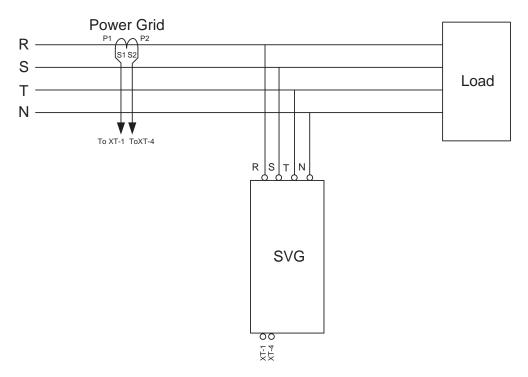
(Figure 3-16: Basic CT Installation and Wiring Diagram\_3)
