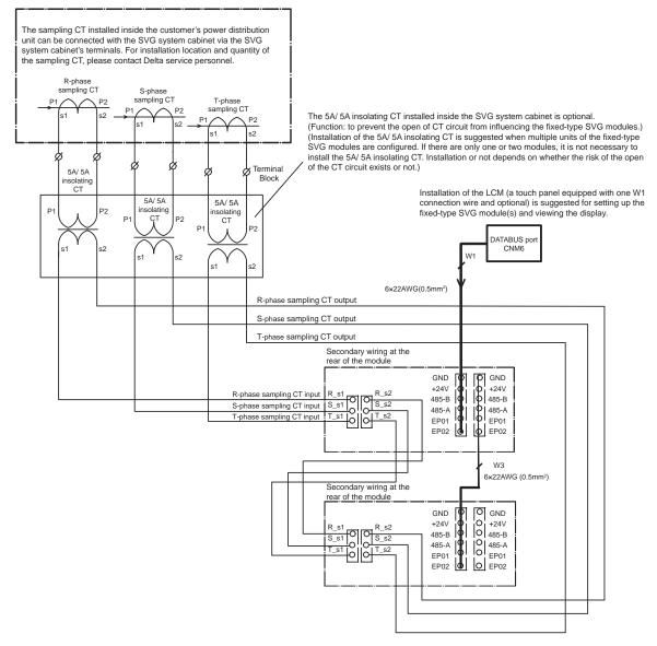
(Figure 3-10: Wiring Connection among the Rear of the Fixed-type SVG Modules, the LCM and the CT)
