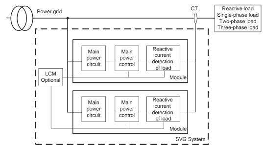
(Figure 2-1: SVG System Block Diagram)
