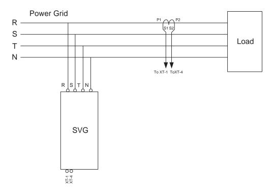
(Figure 3-17: Basic CT Installation and Wiring Diagram\_4)
