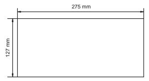
(Figure 3-6: Mounting Hole Dimensions of the LCM)
