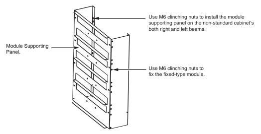
(Figure 3-11: Fixed-type SVG Module Installation Step 1)
