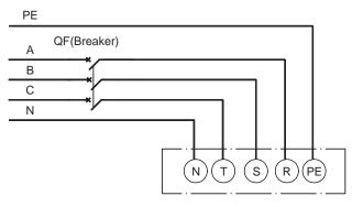
(Figure 3-7: Connection Diagram of Main Power Lines on Rear Panel of the Fixed-type SVG Module)
