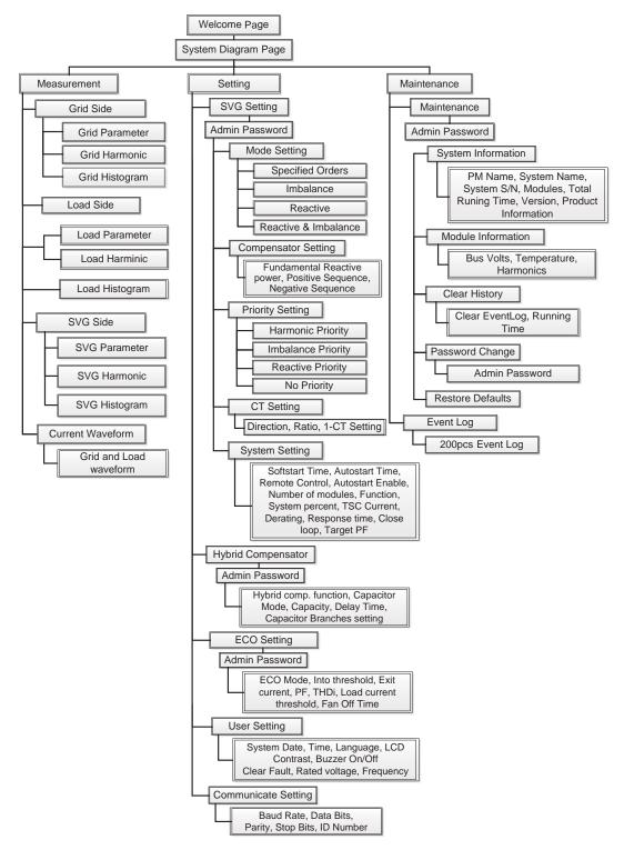
(Figure 5-2: LCM Display Hierarchy)
