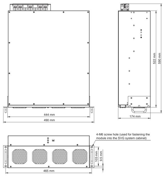
(Figure3-4: Installation Dimensions Diagram\_ Fixed-type SVG Module)
