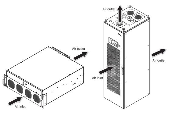
(Figure 3-1: Air Inlet & Outlet Schematic Diagram of the Fixed-type SVG Module)
