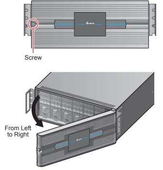
(Figure 3-2: Open the Front Panel)
