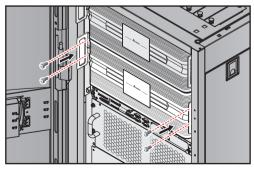
(Figure 4-2: Fasten the Screws)
