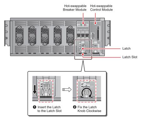
(Figure 4-9: Lock the Hot-swappable Breaker Module's Latch Knob)
