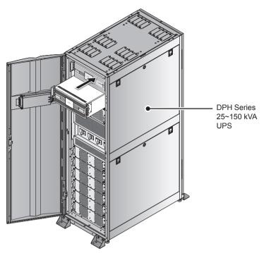
(Figure 4-1: Insert the Rack-mount PDC)
