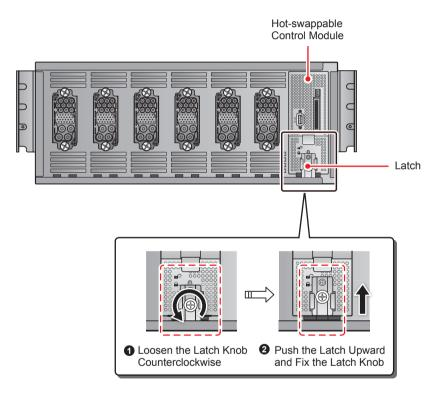
(Figure 4-6: Loosen the Latch Knob, Move it to the Upper Position and Fix it Firmly)
