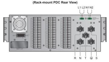
(Figure 5-1: Wiring Terminals\_ Input)
