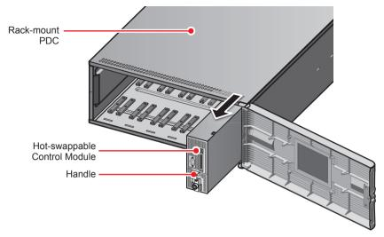
(Figure 4-7: Pull out the Hot-swappable Control Module)
