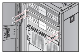
(Figure 4-5: Unscrew the Screws)
