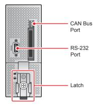
(Figure 4-4: Hot-swappable Control Module)
