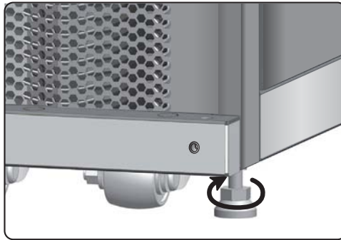
(Fig. 3-3: Rotate each leveler clockwise)
