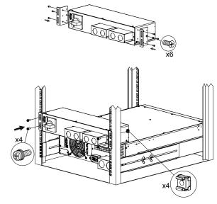
(The screws and cage nuts are provided with the rack frame.)
